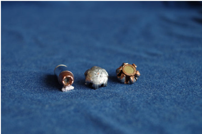
FIG. 5—A “live” (left) and a used, fully mushroomed (center and right) hollow point bullet.
