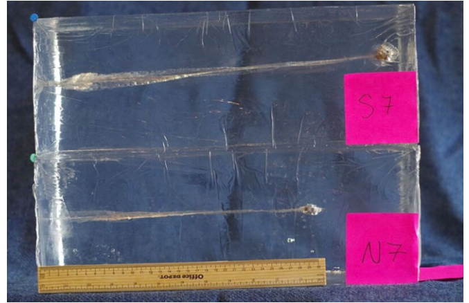
FIG. 3—A representative pair to demonstrate bullet penetration into ballistics gel without (S7) and with (N7) an implant.
